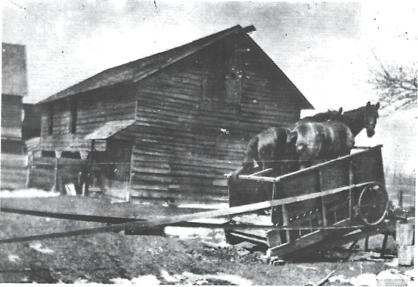
Horse treadmill for threshing at John Van Epps, 1905.
