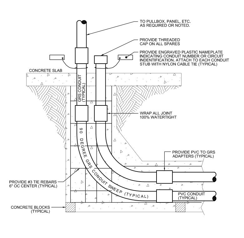
Conduit Stub-Up Detail E-501 SCALE: NTS
