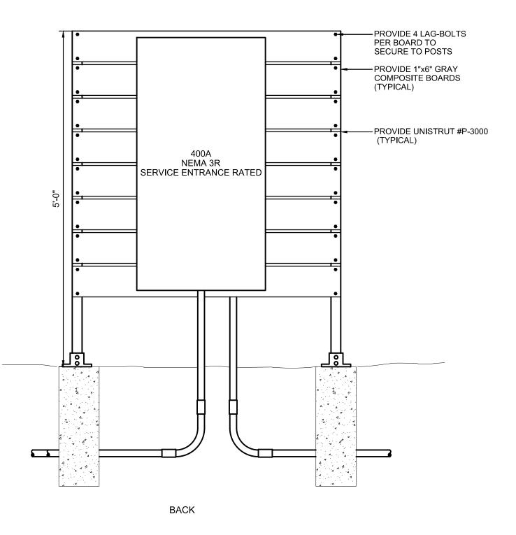
A. ALL OPENINGS FOR CONDUITS SHALL BE MADE IN FIELD ACCORDING TO CONDUIT SIZES AND QUANTITIES.
