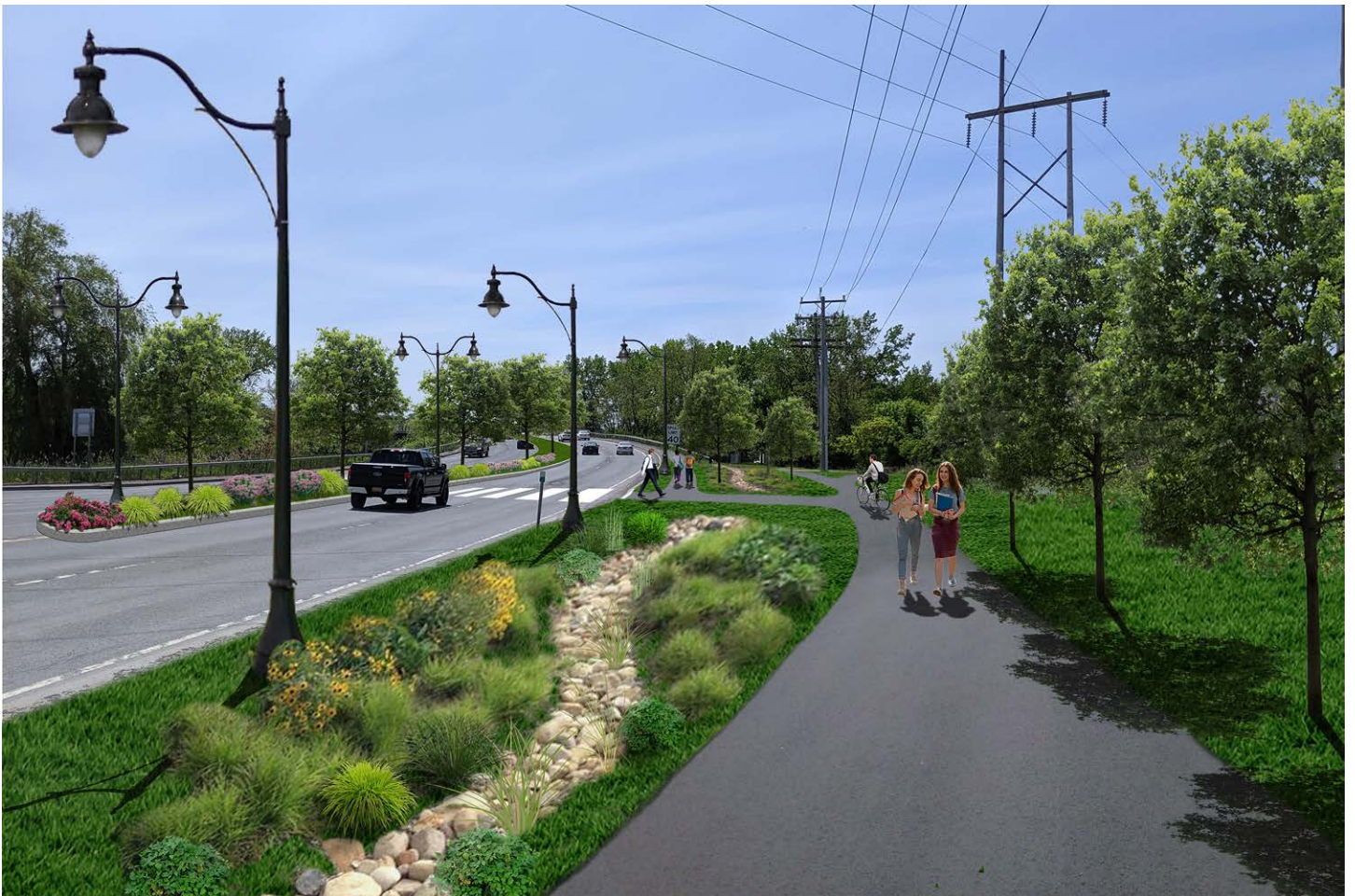
Figure 7. Photo simulation of proposed multi-use path design and stormwater improvements along Freemans Bridge Road.
