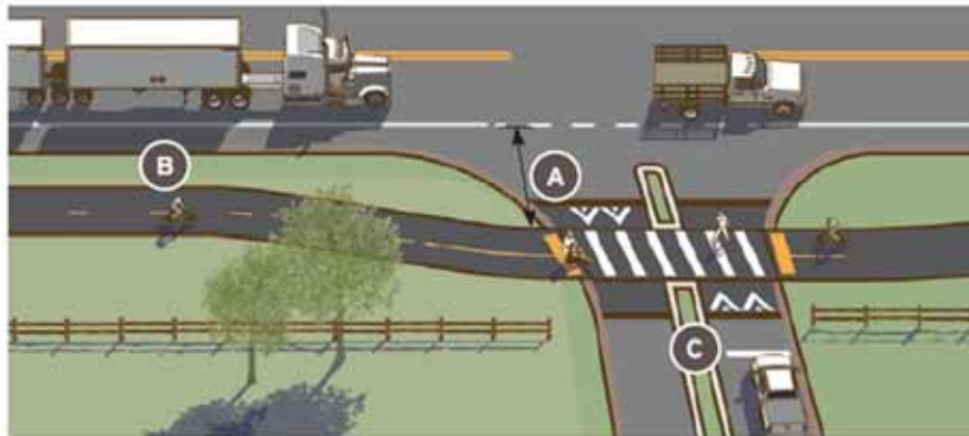
Figure 4-11. Separation distance should be selected in response to speed and traffic intensity. The pathway may need a shift in horizontal alignment in advance of the crossing to achieve desired separation distance. As speeds on the parallel roadway increase, so does the preference for wider separation distance.
