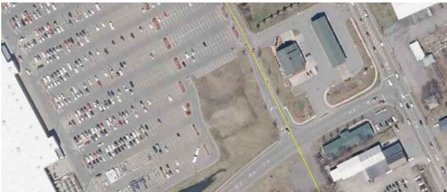
Example of where a hybrid or frontage-type road could be located to provide alternative access off Freemans Bridge Road.
